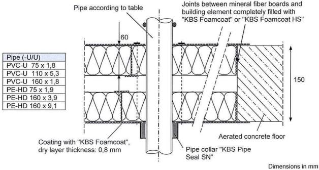
Use as part of mixed penetration seal "KBS Pipe Seal" (El 90)
